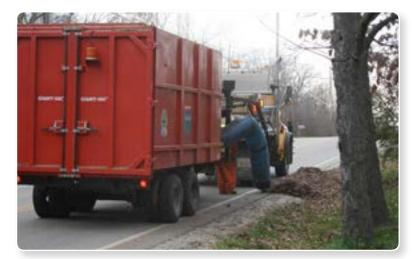
The image above shows how crews use a vacuum to collect loose leaves. Please follow the guidelines to the left to help prevent damage to the leaf vacuum and to make collection as effective as possible for all.
